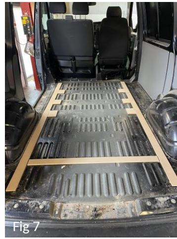
Fig 7 – This shows how the packers need to be placed for the fitting of RIB GlideMotion 150cm
