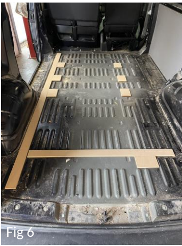
Fig 6 – This shows how the packers need to be placed for the fitting of RIB GlideMotion 112cm
