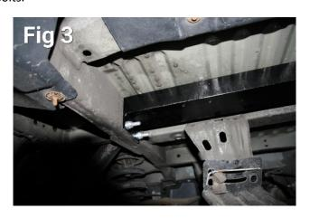
The blind bolts are inserted into the 10m holes one at a time and tightened up. (they require a tap with a hammer to engage) Make sure you use 2 x M10 washers on the behind each nut.
